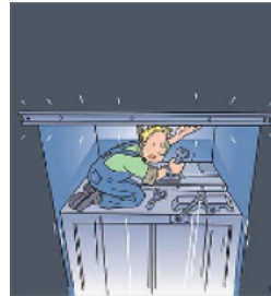
Risk of being crushed on top of the hoistway if insufficient space on the top of the hoistway.
