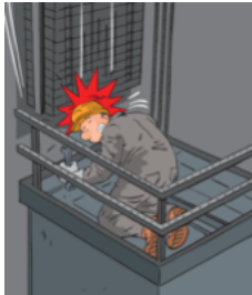
Risk of being crushed by an equipment when moving the car in the hoistway (counterweight, Bracket, etc.).
