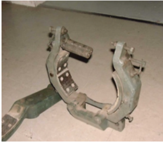
Asbestos in brakes – risk of severe health effects if brake lining are removed without precautions.
